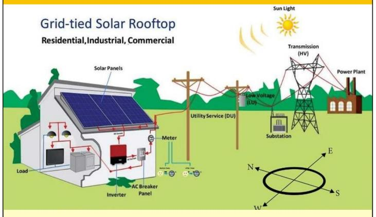
A Grid Tied Solar Rooftop Photo Voltaic (SPV) power plant consists of SPV Array, Module Mounting Structure, Inverter consisting of Maximum Power Point Tracker (MPPT), Controls & Protections, Interconnection Cables and Switches.
